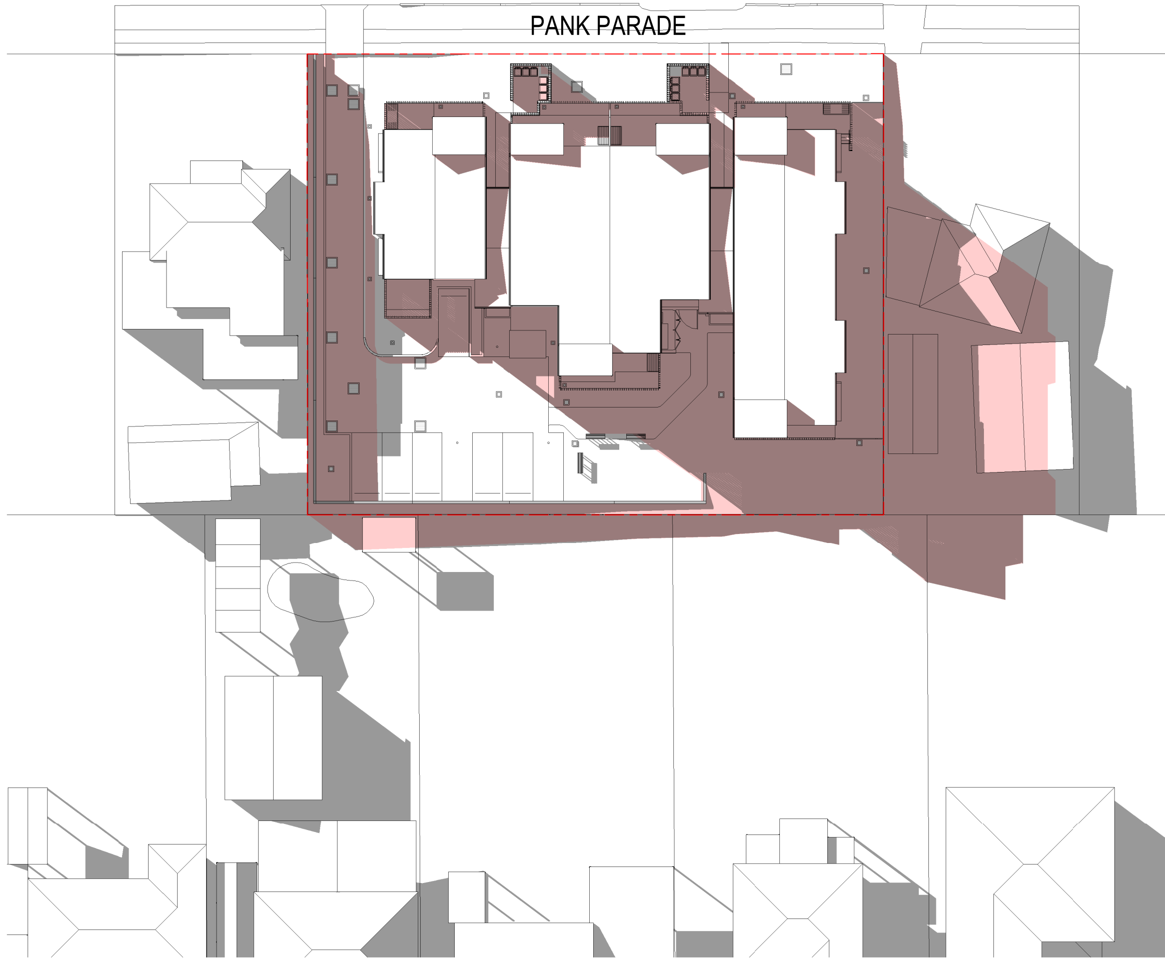
3 3D VIEW SOLAR DIAGRAM - 21ST JUNE 3PM Scale: NTS
